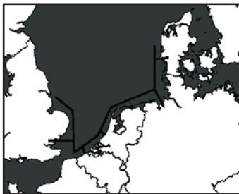
Figure 12-6: Possible first stage of a transnational offshore grid [Shaw 02]
