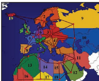
Figure 12-7: Schematic representation of potential electricity transmission paths for an intercontinental overlay transmission system [Czisch 04]
