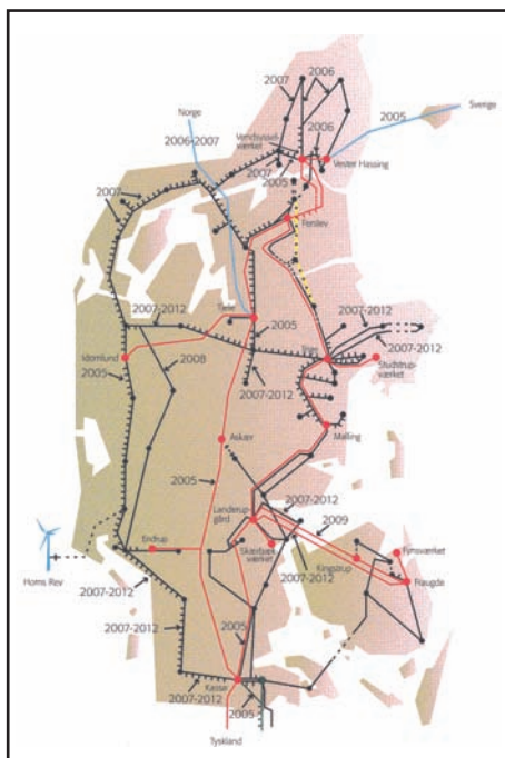
Figure 4-2: Transmission system in Western Denmark (red: 400 kV, black 150 kV, blue: HVDC) [Eltr 04b]
