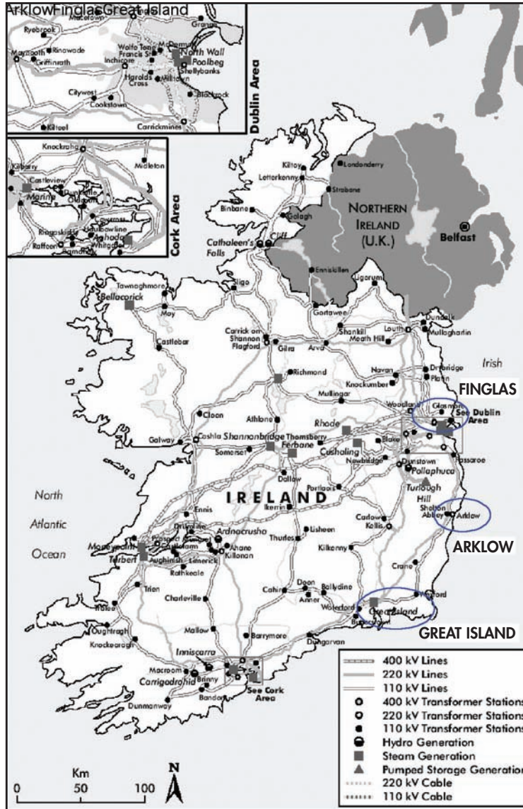
Figure 6-2: National transmission grid with 220 kV substations at the east coast (source EirGrid, from [IEA 04])
