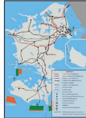
Figure 4-3: Transmission system in Eastern Denmark and areas for existing (green) and future (orange) offshore wind farms [Elkr 04]
