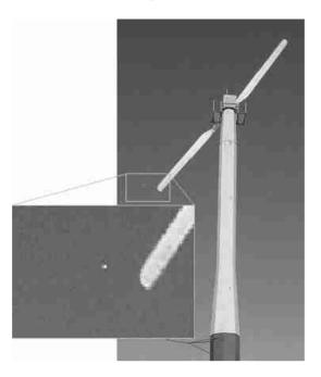
Fig. 6: Tennis ball flies against the rotor blade; the tennis ball is enlarged.
