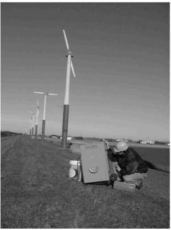
Fig. 5: Tennis ball machine used to simulate bird collisions against the blades
