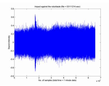
Fig. 7: Sound registration of two tennis balls against the rotor.
