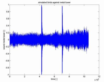
Fig. 4: Sound registration during simulated bird collision against a wind turbine mast.
