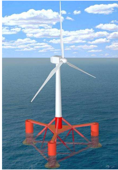
Figure 2: Drawing of the floating foundation construction; design by MSC – Marine Structure Consultants).
