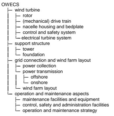
Figure A-2: Components of the OWECS sub-systems
