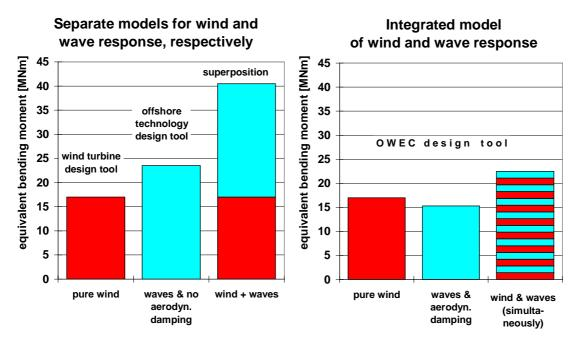
**Figure 7:** Reduction of calculated fatigue loading due to integrated modelling of wind and wave response (right) with respect to superposition of separate models for wind and wave response, respectively (left)
