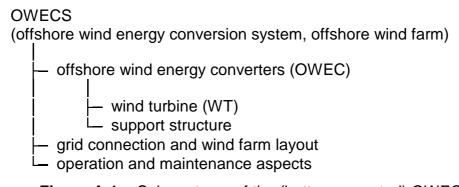
Figure A-1: Sub-systems of the (bottom-mounted) OWECS
