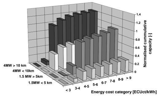
**Figure 9:** Distribution of proportion of installed capacity available at or below particular cost levels employing 100 turbines of 1.5 MW compared to wind farms with 100 units of 4 MW in Belgium and Dutch waters (Values normalised with total capacity employing 1.5 MW units further than 5 km from shore.)
