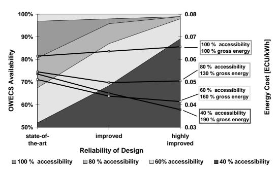
**Figure 5:** Qualitative relation between site conditions (accessibility and gross energy yield) on one hand and availability respectively energy costs for different level of reliability of OWECS design on the other hand
