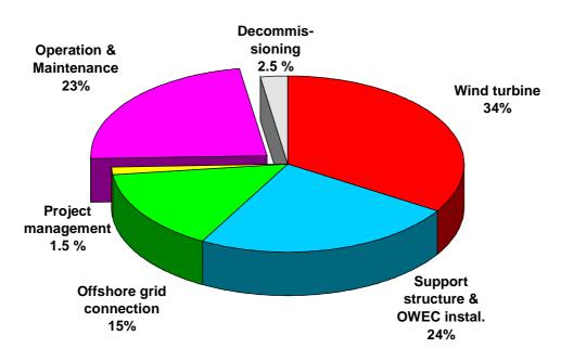
Figure 16: Contributions to energy costs of Opti-OWECS design solution (Annual mean wind speed 8.4 m/s, 20 years loan, 5% real interest rate)
