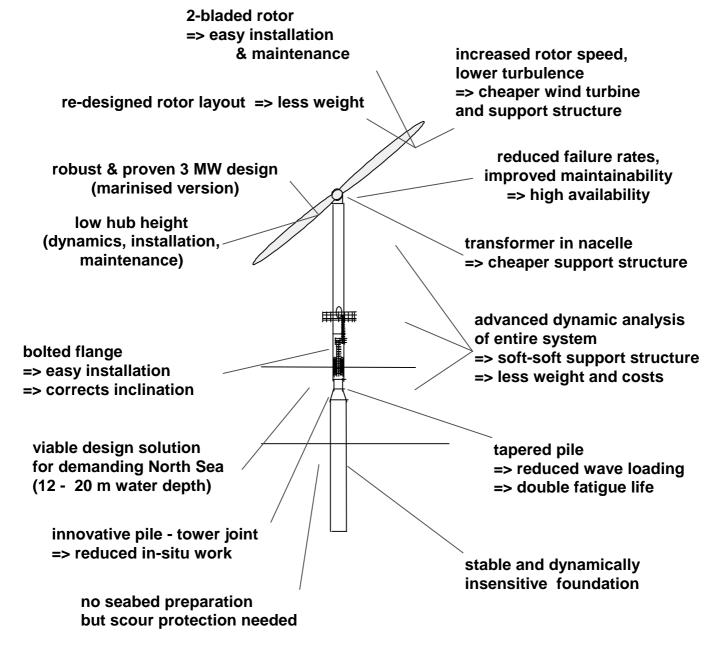
**Figure 1:** Innovative features of the design solution for a 300 MW offshore wind farm (see section 4.4)
