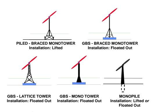
Figure 13: Examples support structure concepts (Concepts in the lower row considered for conceptual design. GBS: Gravity Based System.)
