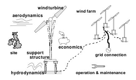
**Figure 2:** Components and aspects of an Offshore Wind Energy Conversion System (OWECS)
