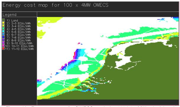
Figure 12: Energy cost map for OWECS employing 100 \* 1.5 MW units (above) respectively 100 \* 4 MW units (below) in Belgian and Dutch waters (Energy cost without onshore grid connection, for 20 years loan and 5% real interest rate.)
