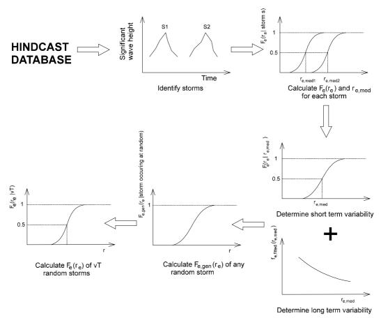
**Figure 6:** The determination of the extreme response distribution with a desired return period based upon the structural reliability method
