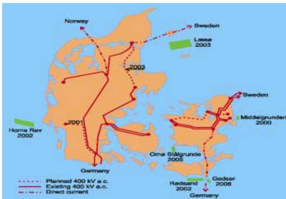
Fig. 3.11: High-voltage grid of Denmark[www.Eltra.dk].
